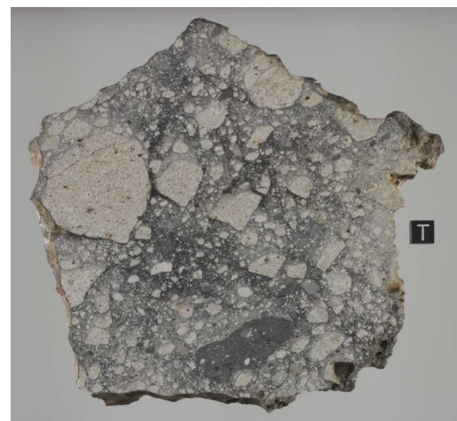
Figure 3: Complete 19 cm slice cut parallel to the top surface shown in Figure 2. Note metal grains with minor rusty staining in leucogabbroic clasts and matrix.
